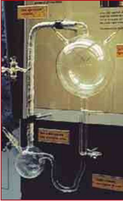
Stanley Miller's experimental setup.
