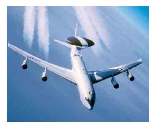
With their highly developed radar equipment, the AWACS (*Airborne Warning And Control System*) in Boeing 767 jets is used for early warning and target control purposes. AWACS, effective in the air and on land, can identify ships on the surface only and fails when it comes to submarines under the water (which are invisible to AWACS). (Bezen Çetin, "Hava Savunma Sistemleri," (Air Defense Systems) *Bilim ve Teknik*, Jan. 1995, 33.)
