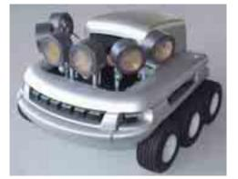
Scientists and engineers have built several robots based on the sonar designs in nature. One of these, the robot named "koala," constructed by the K-Team Company, has six sonar units and was designed for remote-control exploration purposes.
