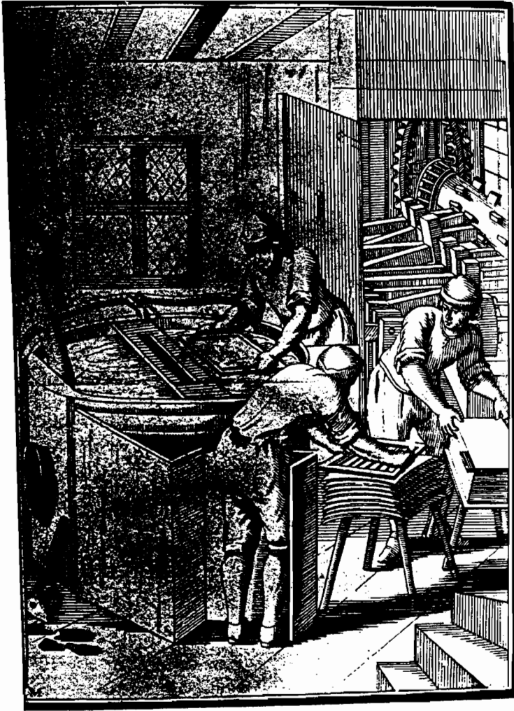
FIG. 147 Papermaking in Europe in the seventeenth century. The vatman, coucher, and layman are performing their respective duties. The "pistolet," or heating device, may be seen at the extreme left of the illustration.
